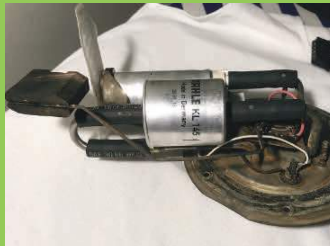
The Pump and Filter with the "tube installed (minus hose clips)
